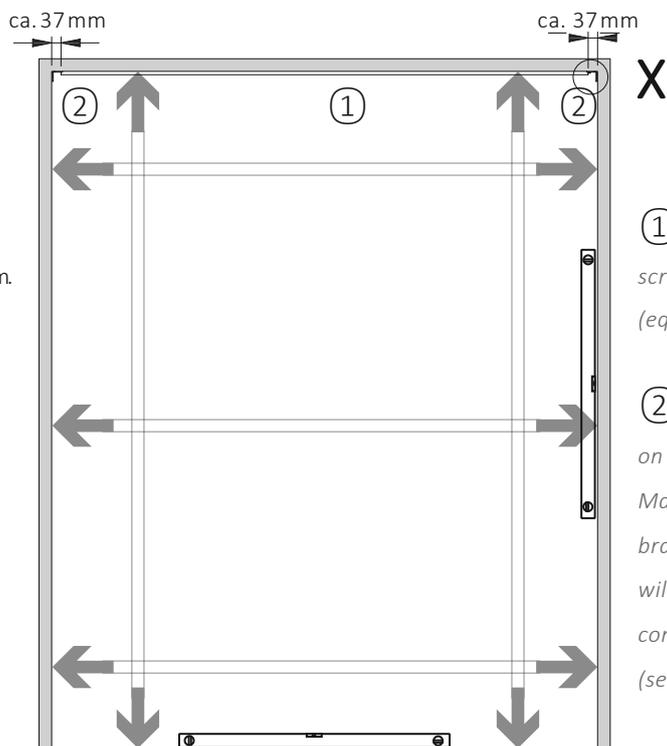
① Wall connection profile screw to the ceiling / lintel (equal distance to both sides).
